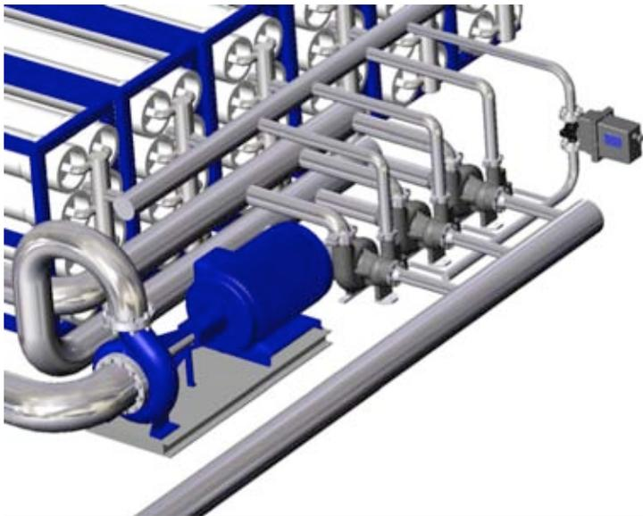
**Figure 13 – ERD center of a 40-50,000 m3/day Three-Center plant using three HPB-960 units**
