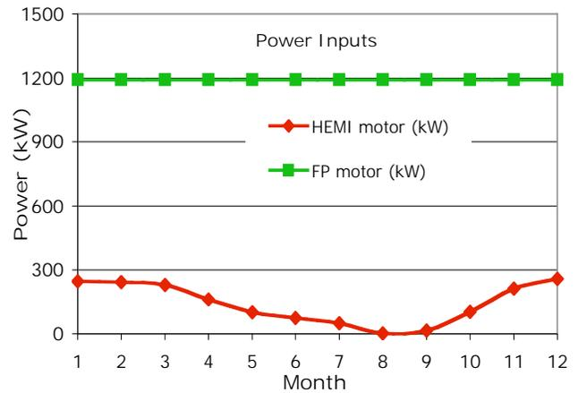
Figure 9 – HP pump and HEMI power consumption
