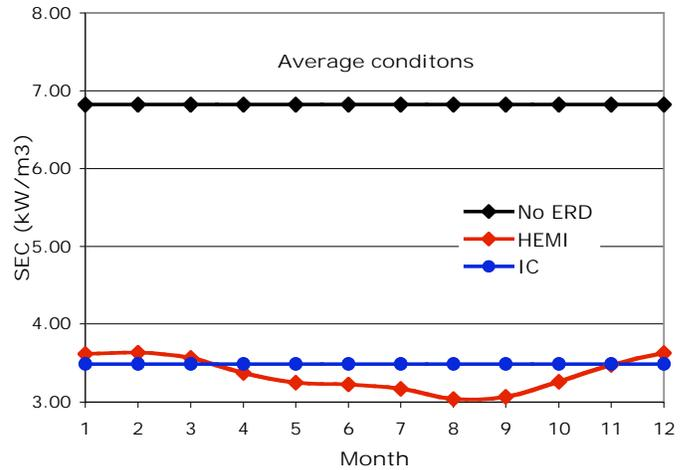
Figure 7 – SEC of HEMI, IC and no ERD
