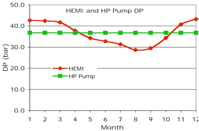
Figure 8 – HP pump and HEMI feed  $\Delta P$
