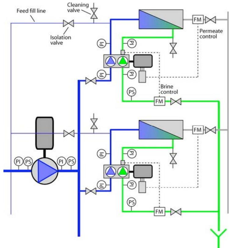
Figure 10 – Hybrid centralization P&ID showing 2 trains
