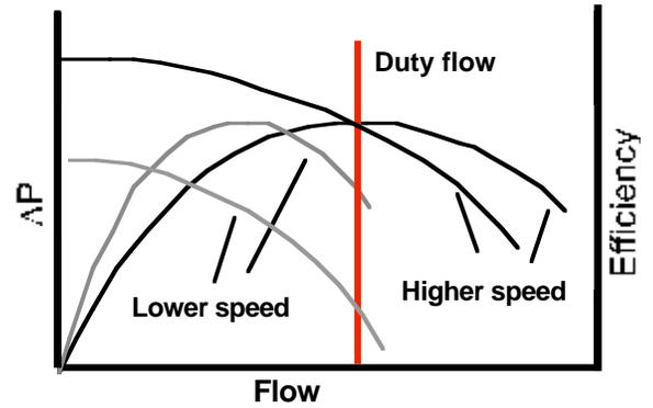
Figure 5 – Effects of large speed changes on pump ΔP and efficiency
