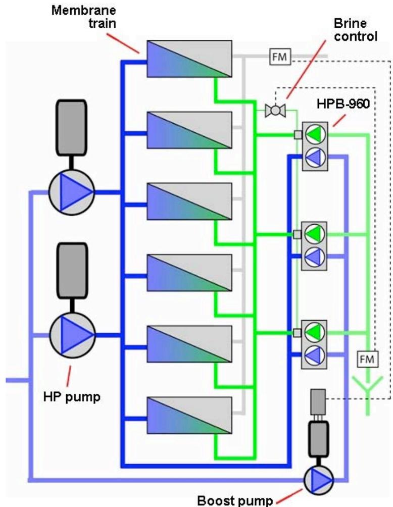
Figure 12 – P&ID for new arrangement of three-center layout
