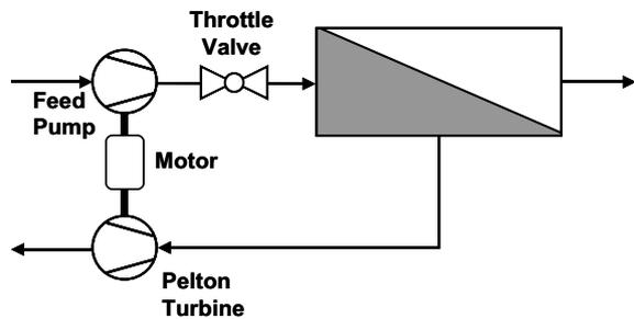
Fig. 2. Feed throttling control, Pelton turbine energy recovery.
