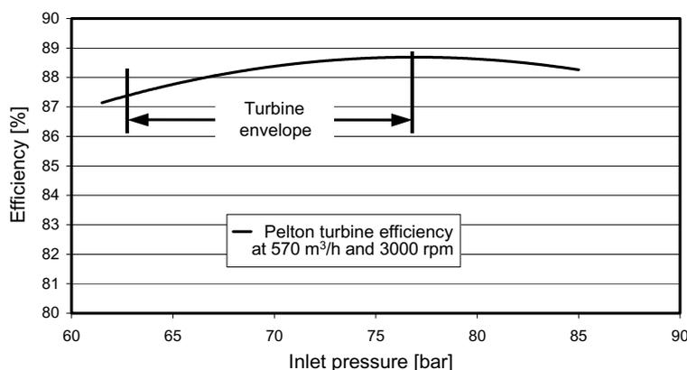
Fig. 8. Pelton turbine efficiency curve.
