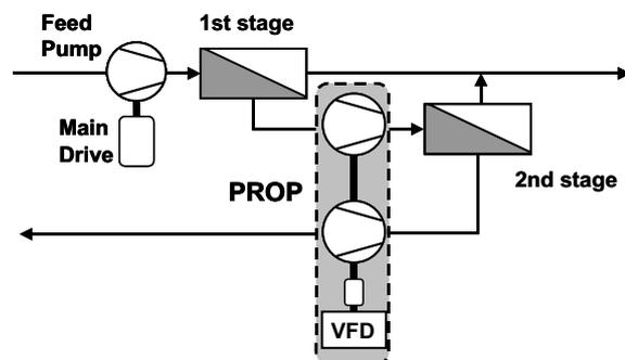
Fig. 7. BCS configuration using the PROP.
