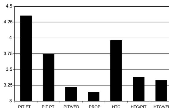
Fig. 9. Specific energy consumption for case study plant — minimum conditions.
