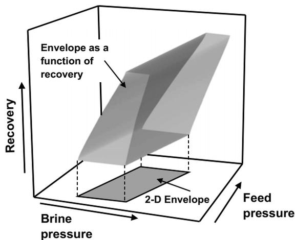
Fig. 1. Three-dimensional hydraulic envelope at variable recovery rate.
