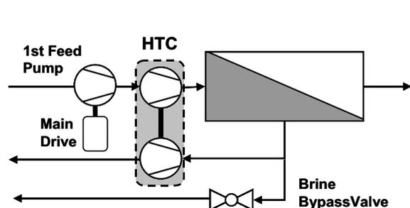
Fig. 4. HTC with brine valve control.
