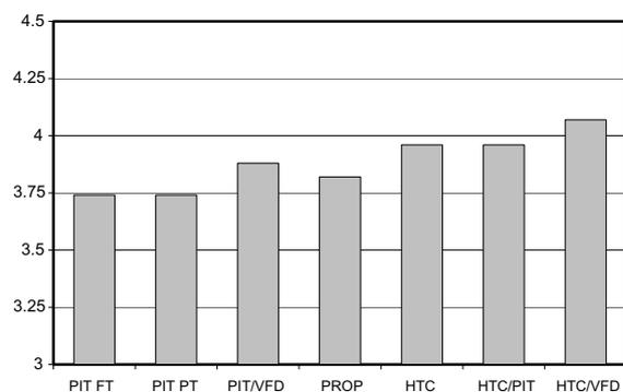
Fig. 11. Specific energy consumption for case study plant — maximum conditions.
