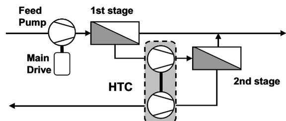
Fig. 6. BCS configuration using the HTC.
