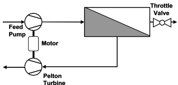
Fig. 3. Permeate throttling control, Pelton turbine energy recovery.
