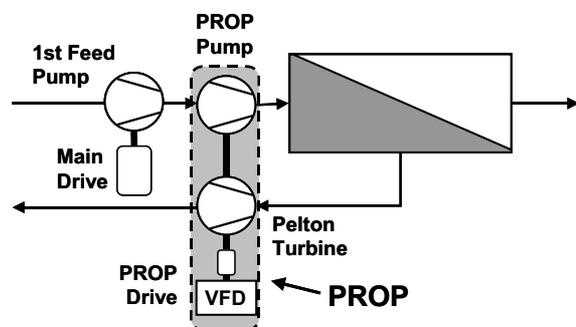
Fig. 5. Control and recovery using the PROP.
